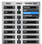
The mentioned information to channel A, B, C and D refer to the speaker output of the GZDSP 4.60ISO. The signal of channel E, F, G and H will be available at the RCA line output (via line out harness).
